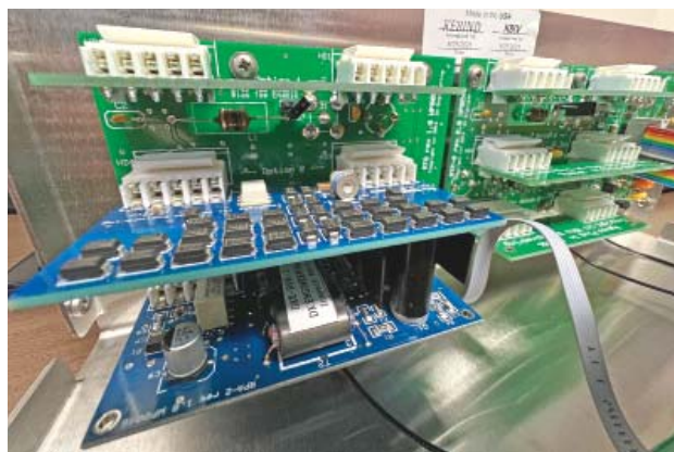
Figure 10 — The NCC-2 internal add-on modules: the DXE-RG5000HD Receiver Guard located in option 2 (middle module on the left side) and the DXE-RPA-2-PM preamplifier module located at the bottom.
