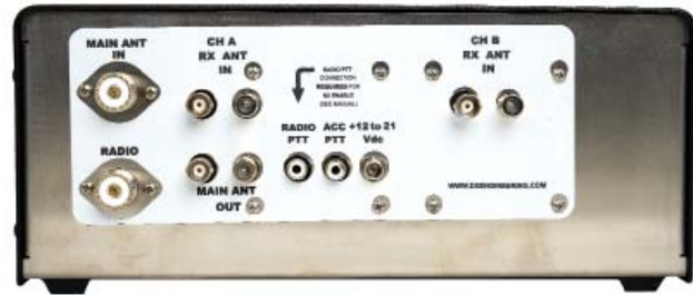
Figure 11 — The NCC-2 rear panel.
