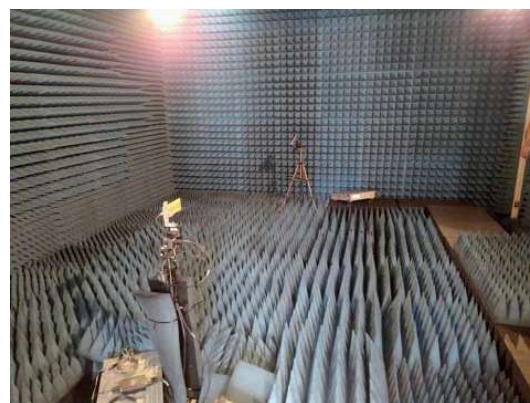
Figure 10. Radiation pattern experimental characterisation setup (a) diagram and (b) photography
