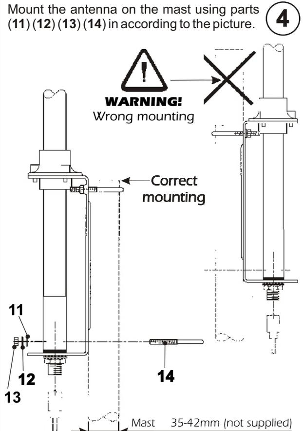
Mount the antenna on the mast using parts (11) (12) (13) (14) in according to the picture.
