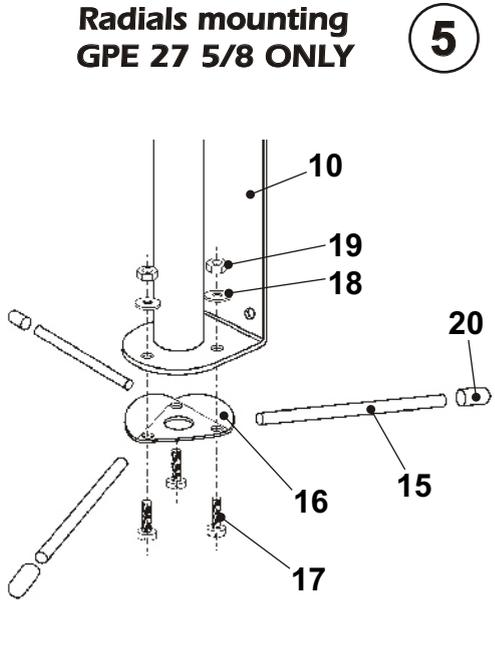
Place the aluminium radials (15) between the steel bracket (10) and the metal plate (16) in according to the picture and lock them by using the supplied screws (17) washer (18) and nut (19). Finally mount the PVC cap (20).
