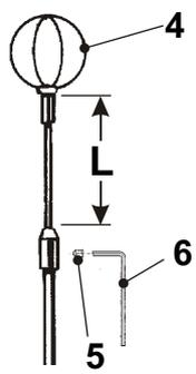
Insert the top section with the cage (4) at L (see tuning table for frequency) and lock it using the screw (5) and 2mm hexagonal key (6).
