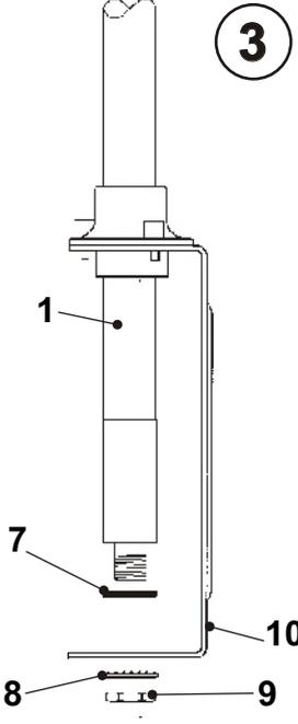
Fit the rubber washer (7) on the bottom of antenna (1). Well lock washer (8) and nut (9) to the steel bracket (10) by using the suitable 19mm key.
