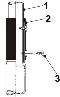
Pull out the sections of telescopic aluminium whip (1), insert the jointing sleeve on the tubes (2) and lock them using the phillips screws (3).
