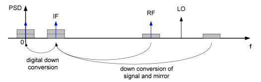
When down converting the RF signal to the intermediate frequency (IF) a double side band mixer is used. It converts both sidebands, the upper  $f_{LO} + f_{IF}$  and the lower
