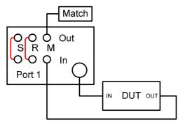
The DUT is connected in such a setup between the normal measurement and the MEAS IN connector of the direct receiver access:
