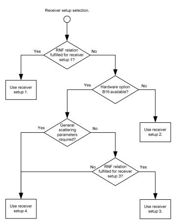
Figure 2: Decision Diagram for Choosing the Receiver Setup.
