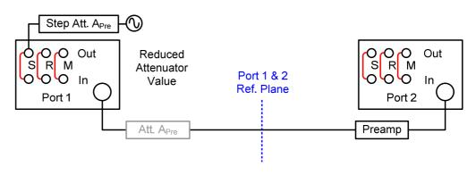
To calculate the noise figure of the DUT correctly, it is necessary to know the noise power, that is applied to the DUT. It is described by the source noise factor  $F_s$  and is measured by connecting the source port with the receiving port without the DUT. In case an external attenuator is applied, use the attenuator value  $A_{\text{Pr}e}$  in this calibration step.
