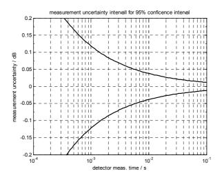
A detector measurement time of 40 ms, with respect to the given figure above, leads to a trace noise of 0.02 dB for the noise power (with 95% confidence interval). If trace noise is not an issue, the detector measurement time can be reduced to smaller values like 10 ms or 5 ms which increases the measurement speed by a factor of 4 or 8 respectively.
