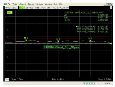
For a complete amplifier characteristic, one might also be interested in parameters like gain, 1 dB compression point or the input or output matching of the device. In a single connection and different channels (see chapter 1.9) the amplifier is characterized in a single shot:
