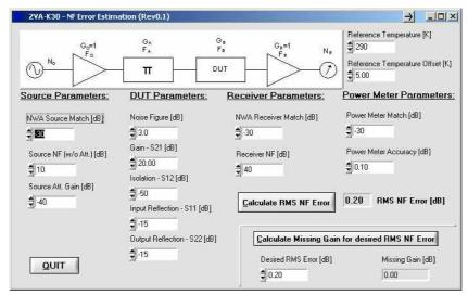
Figure 5: ZVAB-K30 Noise Figure Error Estimation Tool
