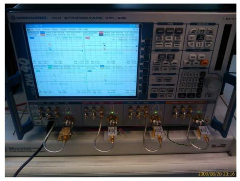
Parallel measurement setup for 4 devices
