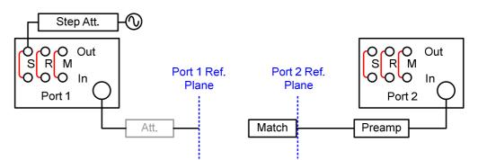
The inherent noise of the receiving port itself is determined during the receiver noise calibration with a 50 $\Omega$  match connected to the receiving port. By measuring the absolute power, the VNA directly calculates the receiver noise factor  $F_R$ . After the calibration step is finished, the receiver noise figure is displayed in the calibration dialog diagram area.
