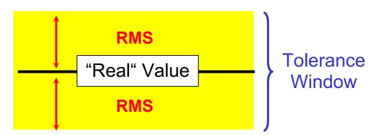
**Application Hint:** In a similar manner tolerances of a noise source  $(\pm 0.2 \text{ dB})$  used for measurement or calibration has to be considered.
