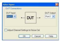
► Select the measurement quantity NF21 with respect to the measurement ports
