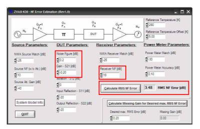
As a matter of fact the expected NF reading for a THRU adapter and a ZVA sensitivity as given in example d) will not show a straight line around 0 dB due to the uncertainty in the measurement setup.
