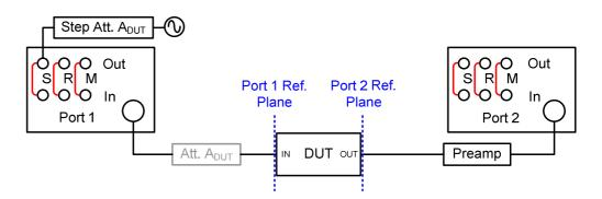
Either internal or external attenuators can be used, depending of their availability and measurement requirements, as discussed in chapter 1.4. However in order to simplify the following description, both internal and external attenuators are shown at the same time. Although uncommon, both types of attenuators could even be used at the same time. The source and receiver reference planes are always assumed to be at the in-and output of the DUT.
