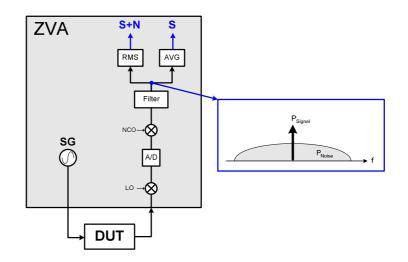
Given a sequence  $x_i$  of complex, filtered, measurement samples (voltages) the VNA calculates the average value  $x_{AVG}$  and the rms value  $x_{RMS}$  value of the samples
