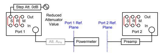
Because the power meter is a broadband device the broadband noise from the VNA source influences the accuracy of the power measurement, especially at low signal levels. For best signal to noise ratio the step attenuator should be set to 0 dB and the port output power should be set to 0 dBm for source power calibration.
