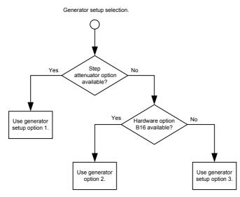
Figure 4: Decision Diagram for Selecting the Generator Setup.
