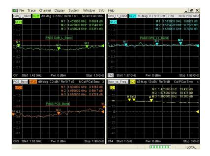
Noise figure measurement in the DAB-L band
