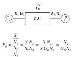
In the above equation S denotes the signal power and N the noise power. At the device under test (DUT) input according to the definition the noise power has to be equal to  $N_0$ . The gain  $G_D$  of the DUT is defined in the context of this application note as the power gain
